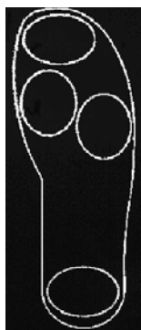
FIGURE 5. Insole with four sensors positioned under the heel and the forefoot.
