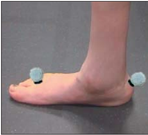
FIGURE 11. An example of two passive markers. They are small retroreflective spheres that reflect the infrared-light.
